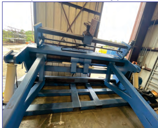
Reel-O-Matic FMP40 Coil Winder (w/ 2-Plane Roll Straightener)
