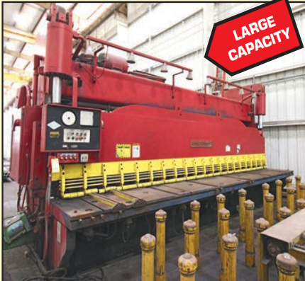
CINCINNATI 20' X 1/2" HYDRAULIC SHEAR
